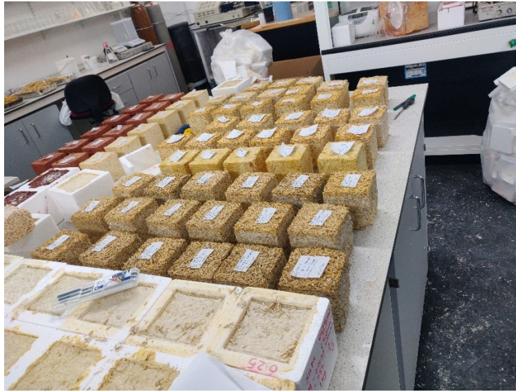
Fig. 16: An image of hemp concrete blocks prepared for compressive strength testing
